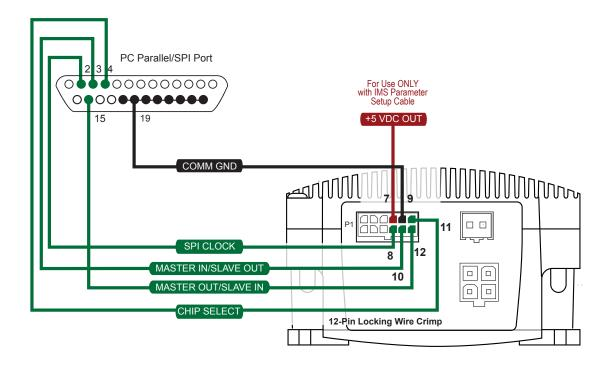
Figure 2.5.2: SPI Pins and Connections, 12-Pin Wire Crimp
